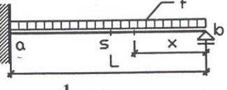
$M_a = -\frac{1}{8} f \cdot L^2$ $\delta_s = \frac{f \cdot L^4}{192 \cdot E \cdot I}$ $x = \frac{3}{8} L$ $M_b = 0$ $M_s = \frac{1}{16} f \cdot L^2$ $M_x = \frac{9}{128} f \cdot L^2$ $V_{ab} = \frac{5}{8} f \cdot L$ $V_{ba} = -\frac{3}{8} f \cdot L$                                                  |
